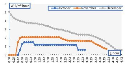
Fig. 4. Dependence of the productivity of the ultrafiltration process of concentrating the extract (extractant-HCl) of orange pectin on the time of ultrafiltration
