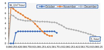
Fig. 3. Dependence of the productivity of the ultrafiltration process of concentrating the extract (extractant-HCl) of lemon pectin on the time of ultrafiltration
