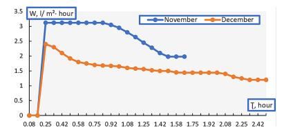
Fig. 5. Dependence of the productivity of the ultrafiltration process of concentrating the extract (extractant-HCl) of pomelo pectin on the time of ultrafiltration
