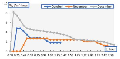
**Fig. 2.** Dependence of the productivity of the ultrafiltration process of concentrating the extract (extractant – HCl) of tangerine pectin on the time of ultrafiltration
