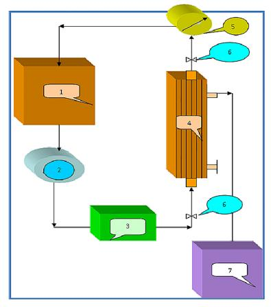
**Fig. 1.** Scheme of the ultrafiltration process: 1 – tank of the initial pectin isolate and concentrate collection; 2 – pump; 3 – mechanical filter; 4 – membrane module; 5 – manometer; 6 – valve for pressure regulation; 7 – container for collecting permeate/
